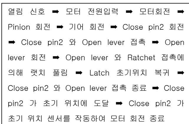
Fig. 4 Open mechanism process
