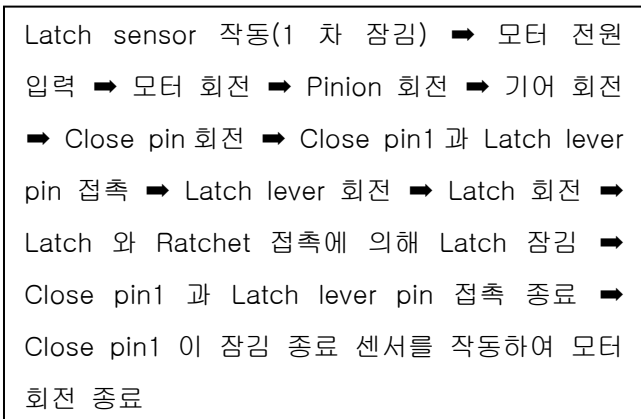
Fig. 3 Close mechanism process
