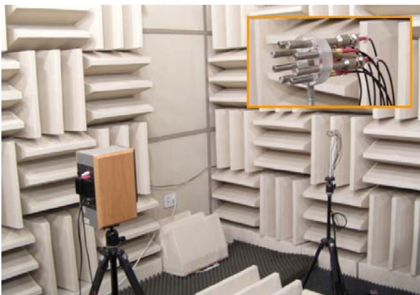
그림 3. Phase Calibration Test at the Anechoic Chamber of Low Speed Wind Tunnel in CNU
