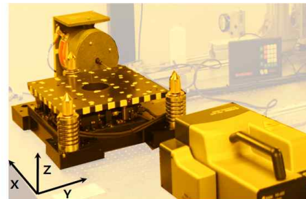
Fig 1. Arrangement of the vibration test for X axis
