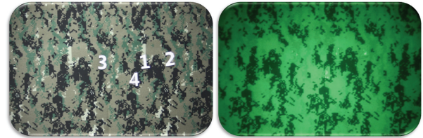
Fig. 4. Near-infrared spectra and Night Vision Devices image of Korean military uniforms.
