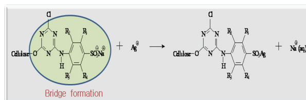
Fig. 3. Process of ion bond between silver nano particle and cellulose fiber treated by Reactive anion agent
