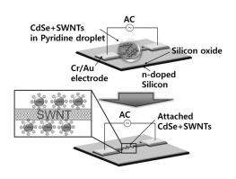
signals from the fabricated aligned SWNTs-FET using dielectrophoresis (DEP), we were able to elucidate the charge transfer mechanism.
