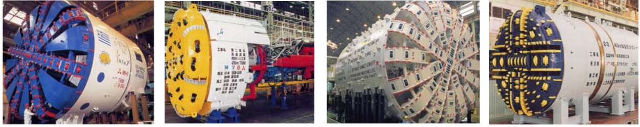
(a) Single Shield TBM (b) Open TBM (c) E.P.B Shield TBM (d) Slurry Shield TBM 그림 1. 각종 TBM 장비
