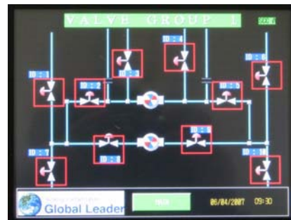
Fig. 10 Detail of main display for sub control console
