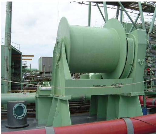
Fig. 16 Picture for spooling device before installation on STP top
