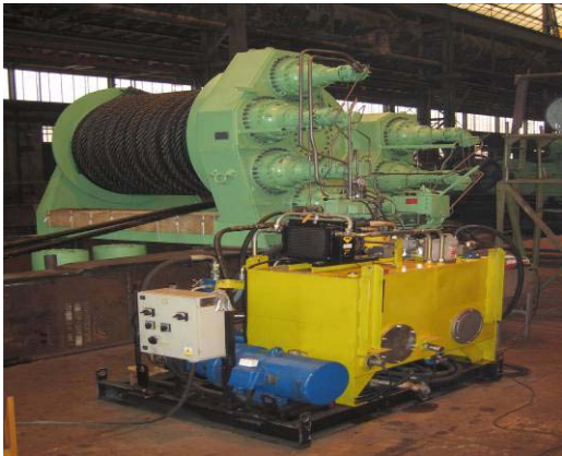
Fig. 15 Picture for Pull-in winch in the shop
