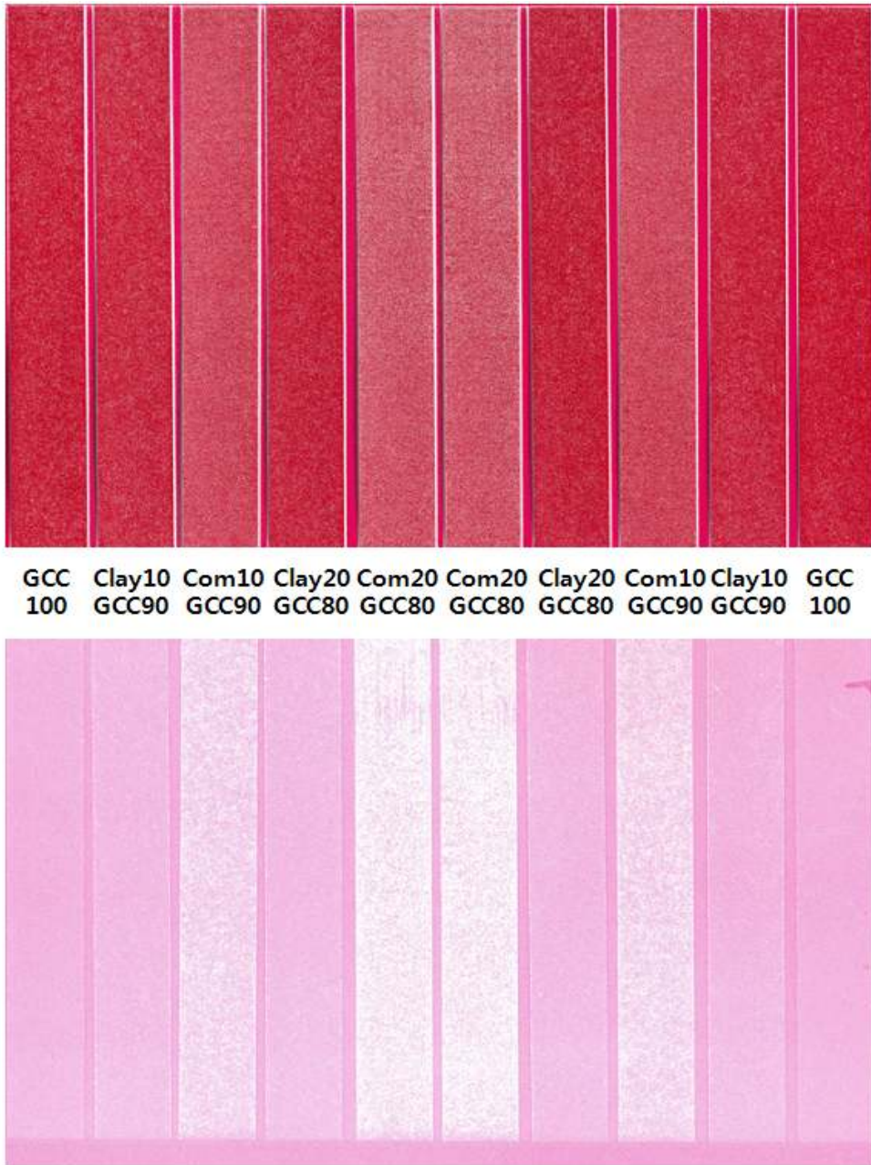
Fig. 6. Dry pick strength of coated paper with ultragloss clay
