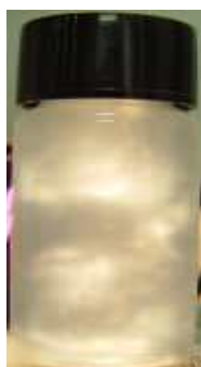
Fig. 5 Flow birefringence of the nanocellulose dispersed in water under polarized light
