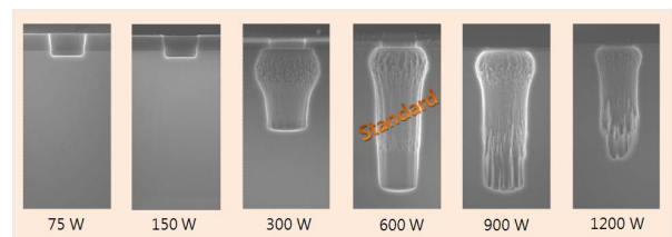
Fig. 3. Silicon deep via formation as a function of ICP power
