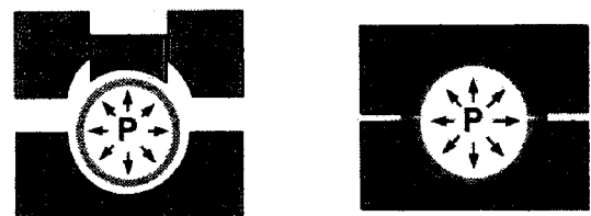
Fig. 1 Hydroforming process for flanged tube parts
