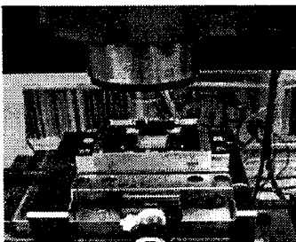
Fig. 7 Micro endmilling system for experiments
