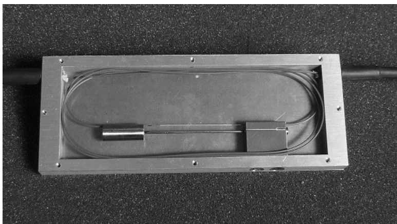
Figure 3. Inner structure of the proto type fiber optic vibration sensor
