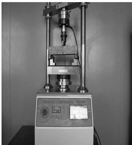
그림 2. Loading frame, and computer for control 3-point bending instrument.
