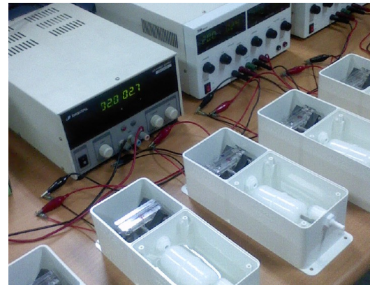
Picture. 1 Performance test of PEM water electrolysis cells
