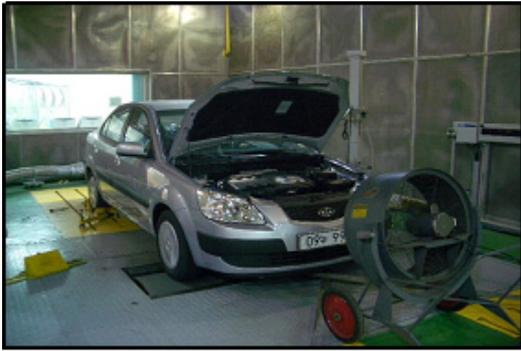
Figure 1. Fuel Economy test for IC Engine
