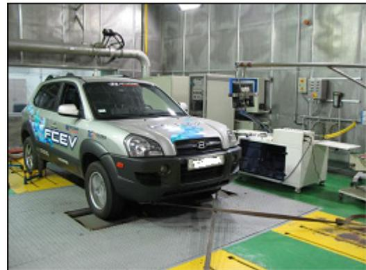
Figure5. Fuel Economy test for Hydrogen fuel cell vehicle
