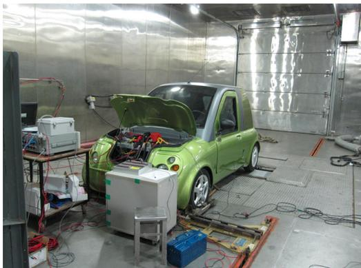
Figure 6. Fuel Economy test for Electricity vehicle
