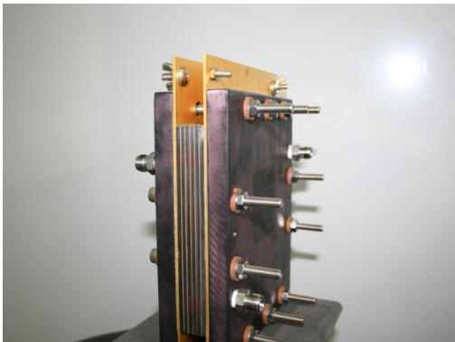
Fig. 1. The photograph of the direct methanol fuel cell composed of five stacks
