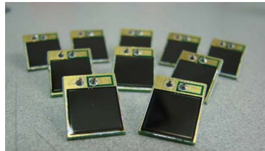
Fig. 1. The fabricated Si PIN-type radiation detector.
