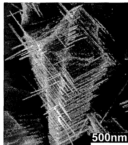
Fig. 1 Manganese nanowires grown from nano particles in 3-D direction
