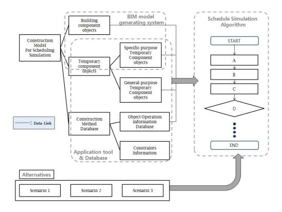
Figure 1. Main elements and the concept model of schedule simulation using BIM
