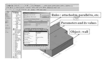
Figure 2. Parametric modeling in BIM tools
