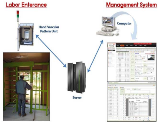
Fig.4. Entity Relation Diagram of Access Management Automation System based on Hand Vascular Pattern
