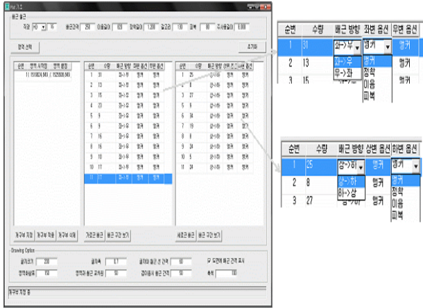
Figure 5. Window for Setting the Foundation Rebar Placing
