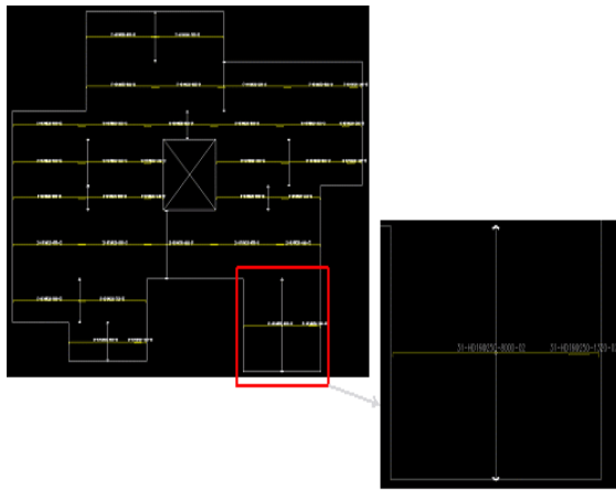
Figure 6. Window for Rebar Placing Around the Foundation
