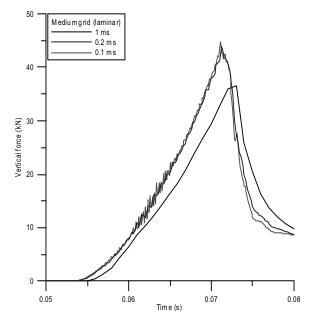
Fig. 7 Comparison of vertical forces (time step size effect)
