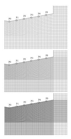
Fig. 2 Three different grid system: coarse (top), medium (middle) and fine (bottom) grid
