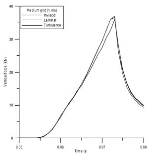
Fig. 4 Comparison of vertical forces (viscosity effect)
