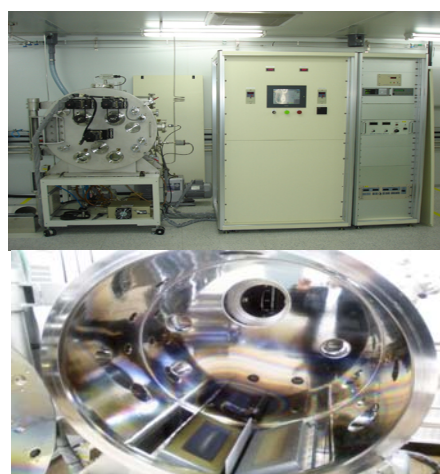
Fig.1. The roll-to-roll sputter system and rectangular cathode used in the AGZO thin film deposition.
