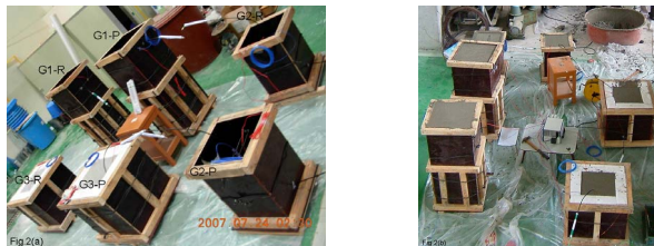
Fig.1 Templates of all specimens (a) before concrete casting (b) after concrete casting
