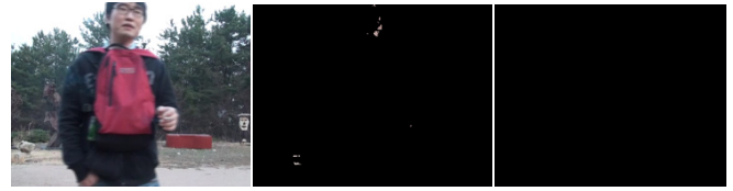
Fig.11 Image with a smoking and moving person on a red bag, the left image is an original image, the middle image is the fire-color processed image and the right one is the result image treated by HMM(without fire)
