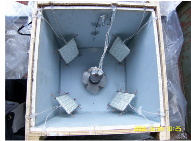
Fig. 2 Slow cook-off experiment layout
