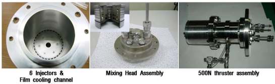
Fig. 5 Fabricated model thruster
