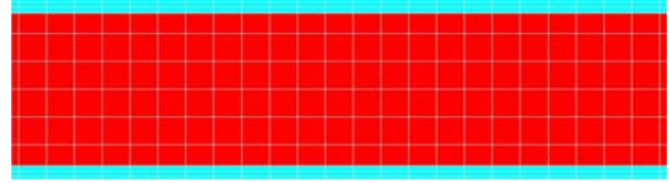
Fig. 5 Grids in steel pipe model.
