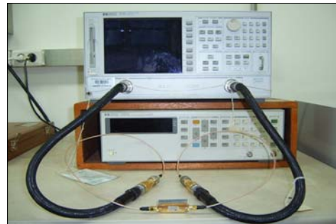
Fig. 11 SAW device measurement setup.
