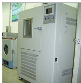
Fig. 10 The constant temperature and humidity controller.
