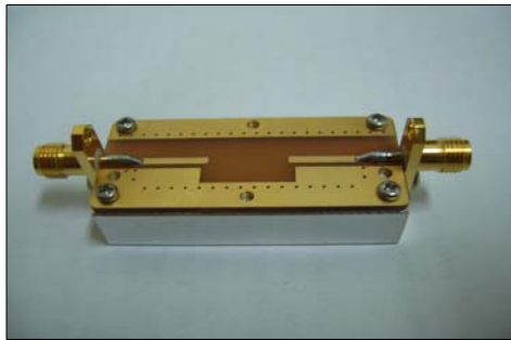
Fig. 8 Photo of test jig for SAW device.
