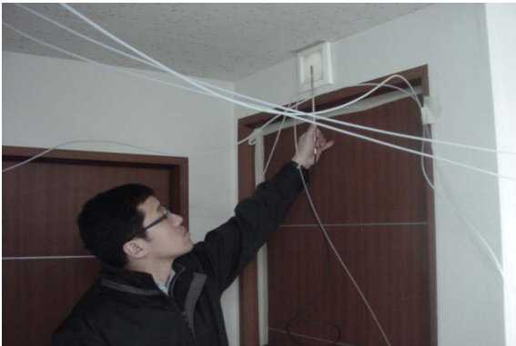
Fig. 9 Photo estimating velocity of air flowing through intervent after enclosing bedroom 2.
