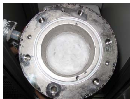
Fig. 3 Photo of methane hydrate in the reactor
