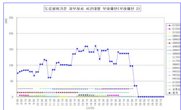
Fig. 3 Expected heating load (Pattern II).
