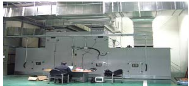
Fig. 3 Experimental apparatus of heat exchanger performance test.
