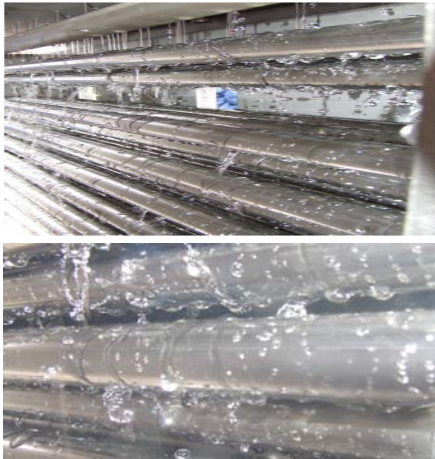
Fig. 4 Flow pattern for velocity=0.6 m/s(mass flowrate is 0.74 kg/s)
