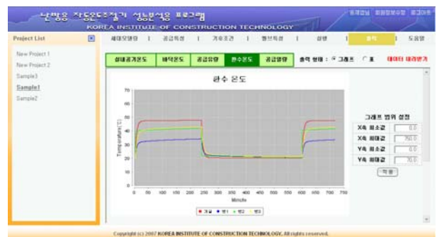
Fig. 5 A output window of return water temperature.
