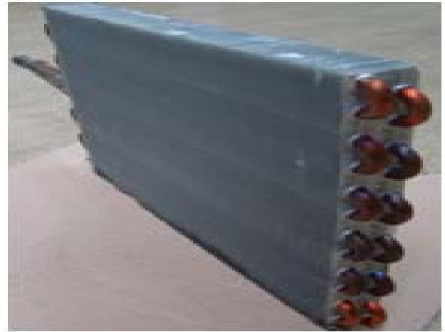
Fig. 2 Shape of test heat exchanger; fin-tube heat exchanger with grooved
