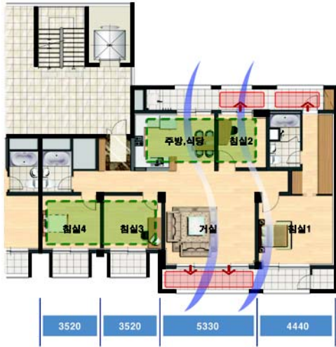
Fig. 3 An unit plan of pilot project building
