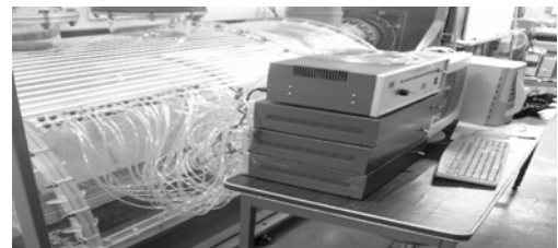
Fig. 6 Pressure Measuring Hole & DAQ System(Data Acquisition System)
