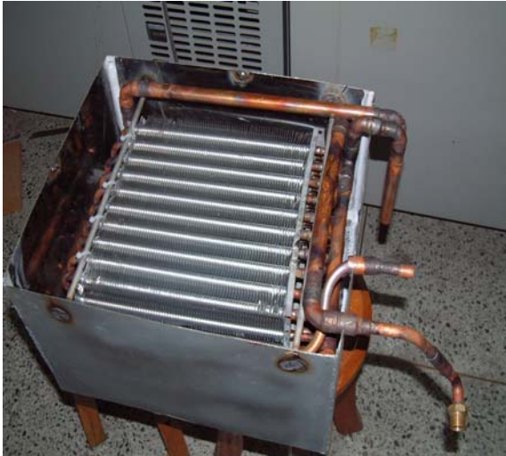
Fig. 3 Heat storage system
