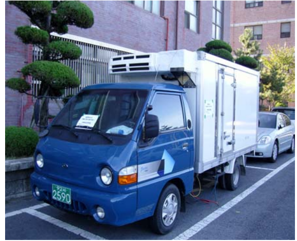
Fig. 4 Refrigerated vehicles of equipped with heat storage
