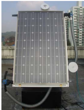
Fig. 2 PVT combined module attached on test Equipment
