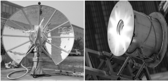
Fig. 1 (a)Dish type solar collector, Inha Dish-1 (b) Solar Chemical Reactor
