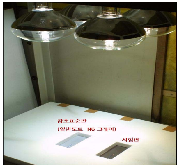
Fig. 16 Experimental setup for measuring the temperature rises due to the radiation
