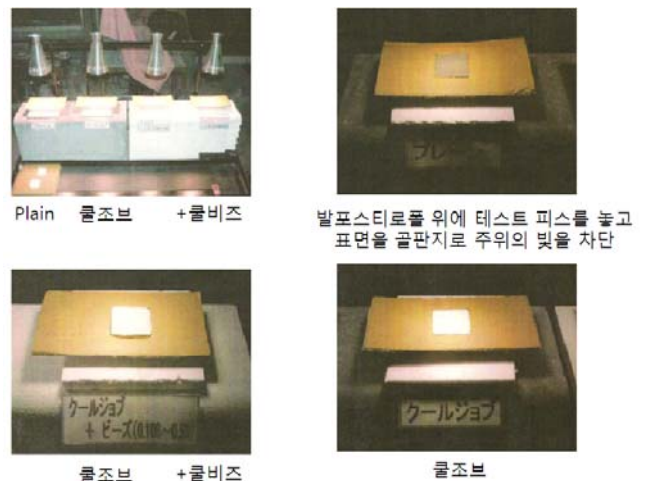
Fig. 5 Experimental conditions for measuring the temperature differences in Road Cooler depending on bead diameters
