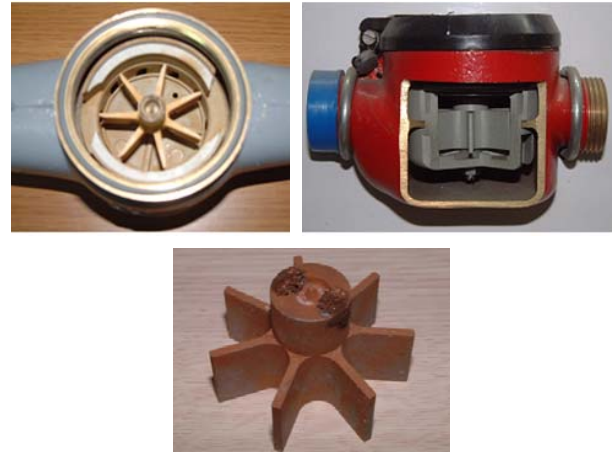
Fig. 1 The structure of impeller type of flow meter and its polluted state after 60 days experiment with muddy water of 2500 NTU.
