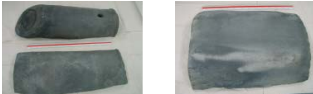
그림 1. (a) Channel tile(upper) and roof tile of the South Gate(lower) (b) Jangheung roof tile
