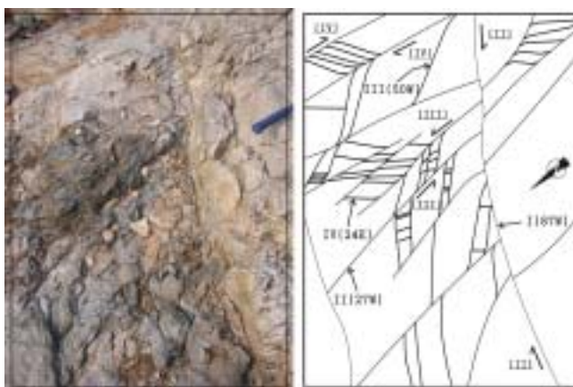
Fig. 4. Outcrop photograph and sketch. Numbers and arrow marks in outcrop sketch refer to the orientation (e.g. 87W) and the relative timing of joints (e.g. I, II) and shear fractures (e.g. II, III), and the sense of shear fracturing
