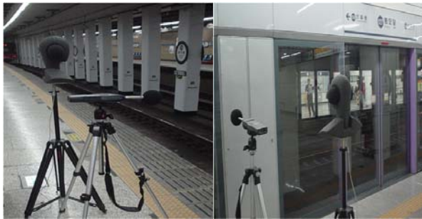
Fig. 1 Noise measurement of subway stations
