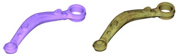
(a) 3D surface model (b) Finite element model Fig. 1 Aluminum upper control arm model
